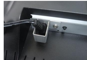
Power plug bracket Keeps power plug in place
